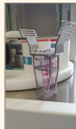
Figure 5 - Presto automated processor/ stainer slide rack showing a six-slide capacity.
