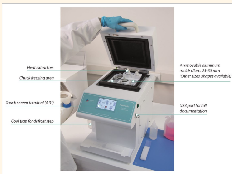
Figure 1 - Key features of the PrestoChill Cryoembedding System
